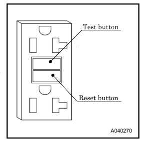
IF THE GFCI CANNOT BE RESET: The GFCI is faulty. Contact your nearest dealer. IF THE GFCI RESETS PROPERLY: Check the appliance or the power cord.
