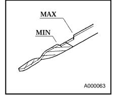
While checking oil level, check also for contamination. If the oil is found dirty, contaminated, or should be changed according to the periodic inspection list, change the oil.
