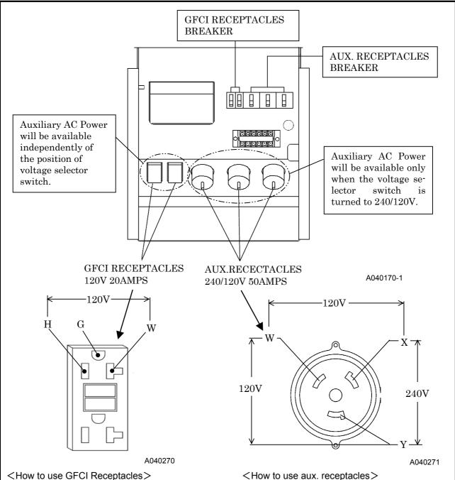
It is available to get 1 phase/120V from GFCI receptacles independently of the position of voltage selector switch on the control panel.
