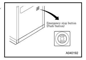
• To reset the button, turn the button head in the direction of the arrow. If it is not reset, the machine cannot restart to operate.
